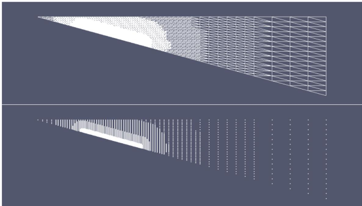
**Figure:** Actual spatial resolution of the simulation (wireframe / vertices as dots)
